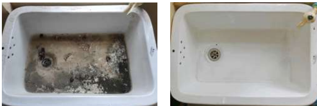
Figure 7. Before and after cleaning of ceramics basin with 50% eco-enzyme
